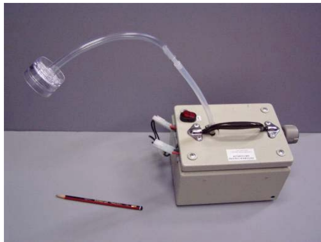
Figure 2. Short duration (10-20 min.) air sampling pump with filter attached
